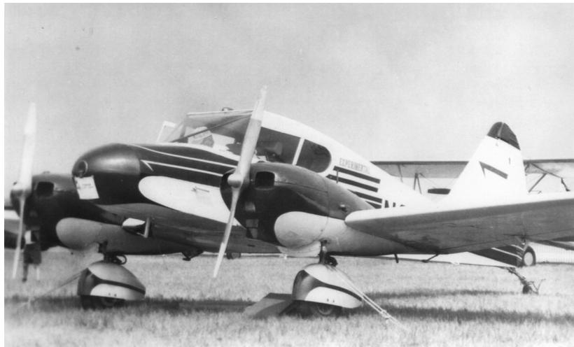
The Langley is a very rare airplane indeed, only about 3 or 4 were built, although it was a Type Certificated airplane, achieving ATC number 755. Built during World War II when aluminum was very scarce, it is a laminated all wood airplane, twin engine with fixed landing gear. Imagine a small looking Twin Beech, complete with twin fins and rudders, and you have a reasonable idea of what the Langley looked like.
